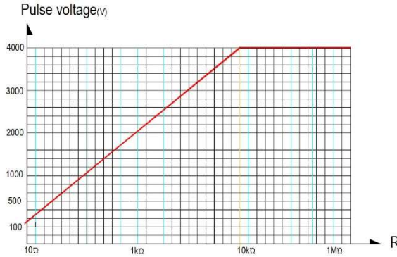
Pulse load rating in accordance with IEC 60115-1,4.27; 1.2µs/50µs ; 5 pulses loaded, for permissible resistance change <\pm(0.5\%+0.05\Omega)
